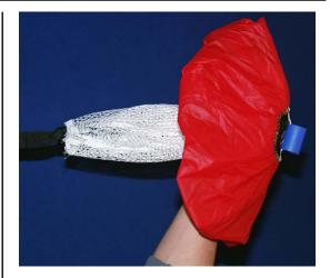
Than put it in the center of the ZeroP fabric and fold the bridle on too.
