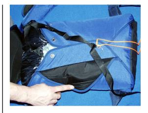
Than close the second loop. Be carefull to rout the bridle in the same way as in the picture.
